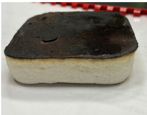
Figure 17. Composite material based on microfibrillar cellulose and fungal melanin
