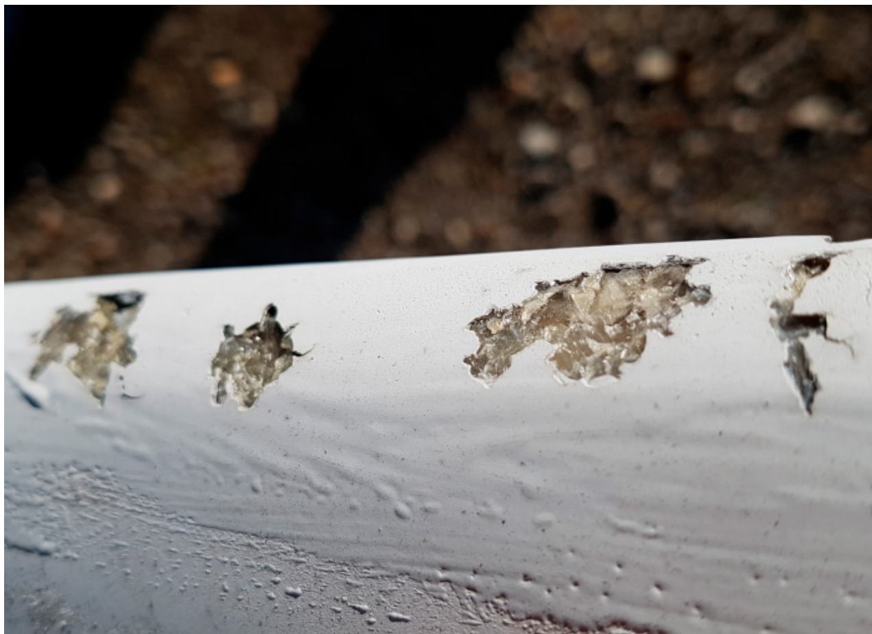
Figure 14. The leading edge erosion of a wind turbine blade
